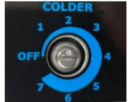
8. **Set the thermostat on EC versions.** Thermostat settings need to be adjusted through the control panel. The default settings are -2 C for the summer months and +2 C for the winter. We recommend you set both to +2C. Please see the instruction manual for programming instructions. Failure to set the thermostat correctly could lead to a frozen ice bank.
